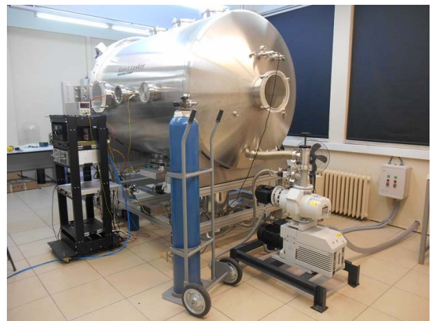
Fig. 4. The picture of the mechanical pump and the roots blower
