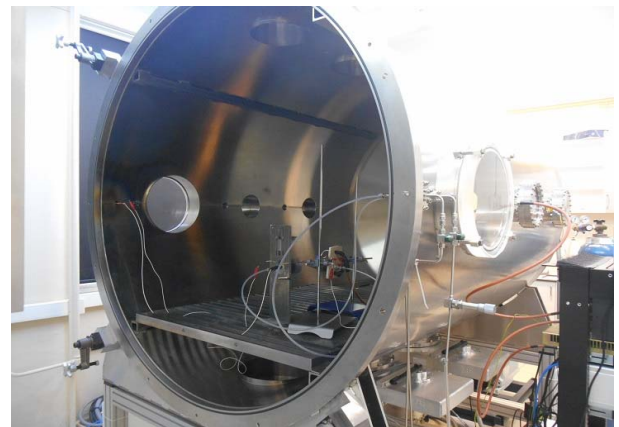
Fig. 8. Pictures of the cusped field Hall thruster and the RF cathode placed on a stand inside the BUSTLab vacuum chamber for testing
